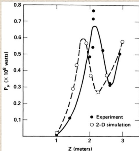
Amplified signal output as a function of length along the undulator. The FEL operates at a frequency of 34.6 GHz, and the input signal, provided by a magnetron, is about 50 kW. From reference [Orzechowski, et al., 1985].
