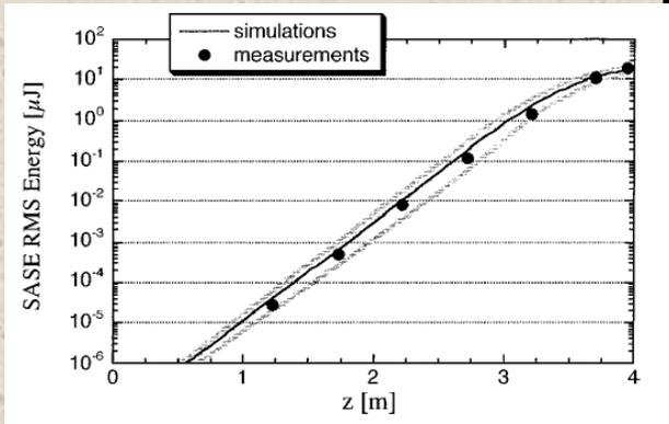
Measured SASE intensity vs undulator length and numerical simulations (gray lines are the rms boundaries of the set of GENESIS runs). The amplification curve yields a power gain length of 17.9 cm and saturates near the undulator exit.  $\lambda =$
