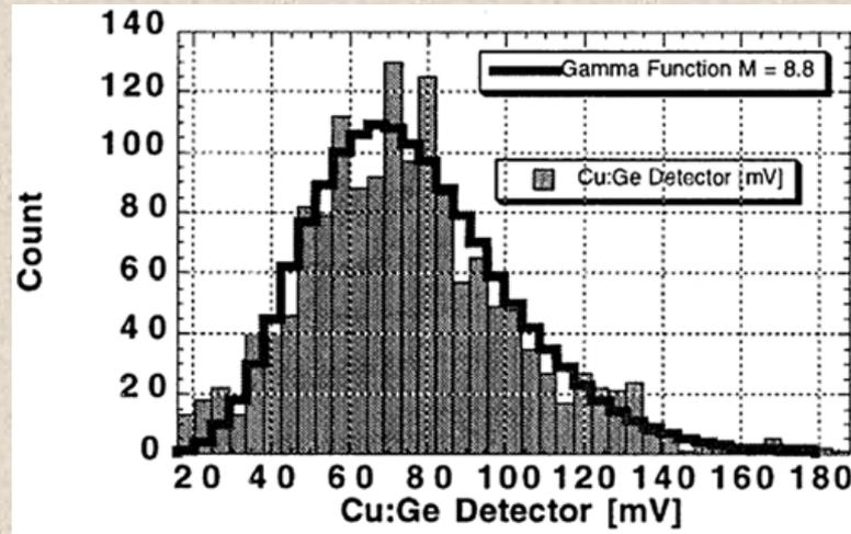
Intensity fluctuations for individual 2 nC micropulses compared with theory.
