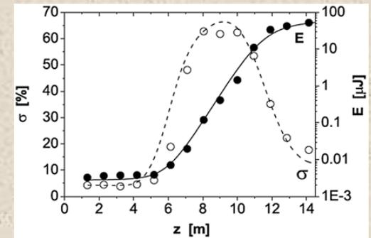
Average radiation pulse energy (solid circles) and rms energy fluctuations in the radiation pulse (empty circles) as a function of undulator length. Wavelength 98 nm. Circles: experimental results. Curves: numerical simulations. Reference Ayvazyan et al. 2002.
