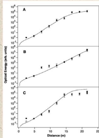
Intensity vs undulator length for various electron beam conditions. (A) 530-nm saturated conditions. (B) 530-nm unsaturated conditions. (C) 385-nm saturated conditions. Solid curves: GINGER simulation results. Reference Milton et al., 2001. G. Pellegrini
